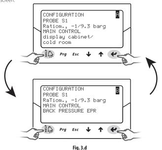
Important: the probe S1 parameter is common to both drivers, while the main control parameter must be set for each driver. See the table of parameters.
