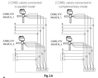
Important: in the case of installations with four valves, the EVD0000UC0 module cannot guarantee all four will close in the event of power failures.
