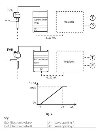
For the wiring, see paragraph "General connection diagram".
